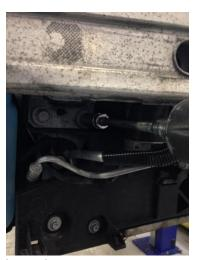
8. Un-clip intercooler on drivers side and slide cooler across
