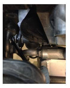
10. Install the intercooler by fitting the N/S first, clip boost pipes on and secure with fittings provided, replace parts in reverse order of removal
