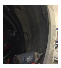
3. Remove 2 x T30 screws securing bumper to wing '1 x each side', then remove x 7 10mm bolts securing bottom of bumper
