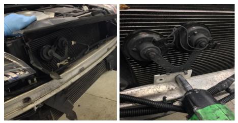
7. Undo 10mm bolt that secures headlight to crash bar and loosen off 16mm bolts for crash bar
