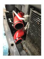
9. Fit intercooler with side brackets attached
