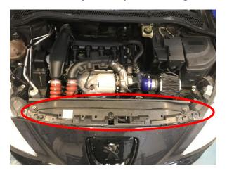
2. Undo 3x 8mm bolts securing top of bumper to wing
