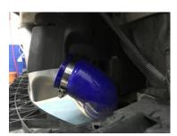
12. Back of bumper grill slight trimming is required to clear intercooler
