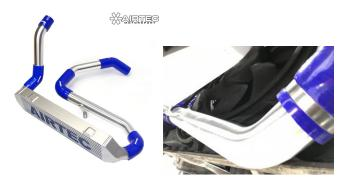
10. Once happy with clearance, tighten bottom boost pipe to intercooler and all jubilee clips
