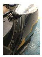
3. Remove 3x plastic push fit fittings on inner arch to bumper
