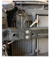
Start by loosely fitting all pipework as numbered below. As a starting point, number 1 to crossover and number 5 to turbo outlet.
