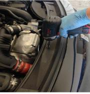
2. Undo T20 Torx and plastic clips securing inner arch to bumper.
