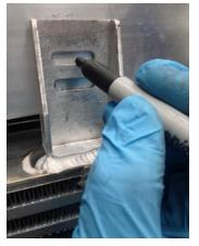
9. Fix intercooler into place with the bolts supplied. Offset bolts slightly to allow clearance for washers.
