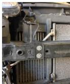
7. Offer airtec intercooler into place, when happy with clearance bolt to radiator front panel with supplied self-tapping bolts
