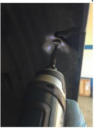
3. Undo 2x 10mm bolts holding bumper to front arch and gently pull the bumper to unclip.
