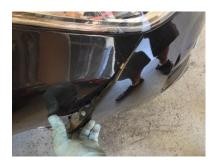
4. Remove bumper making sure to unclip fog lights.
