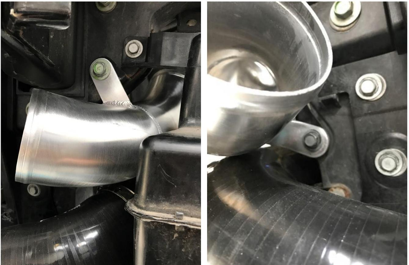
19. Fit the 45-degree silicone joiner to 90-degree MAF sensor hard pipe, as shown. Then attach the silicone joiner to the turbo.
