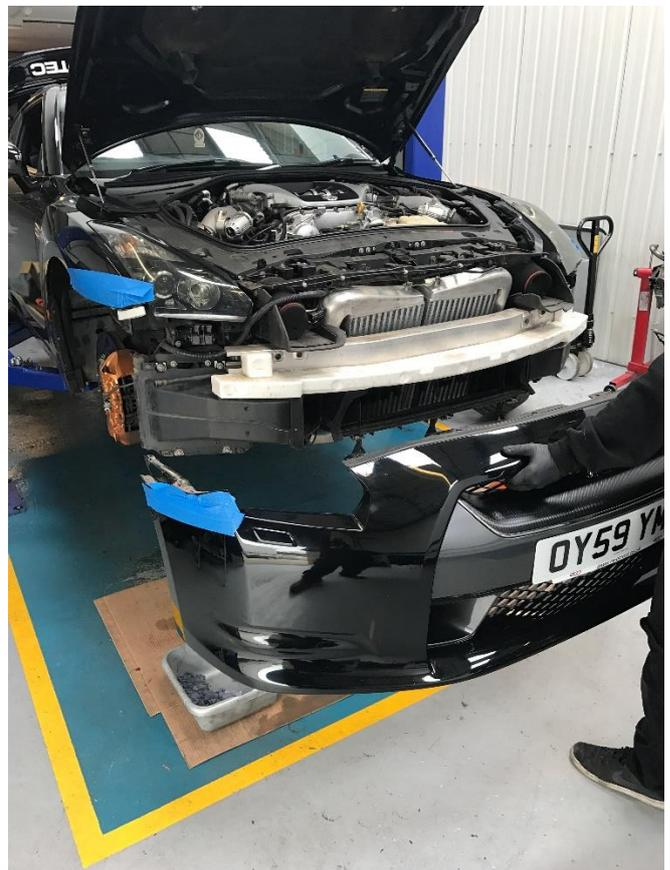
8. Release the eight 12mm bolts (blue arrows) to remove the crash bar, as well as the six 10mm bolts (orange arrows) for the front splitter supports.
