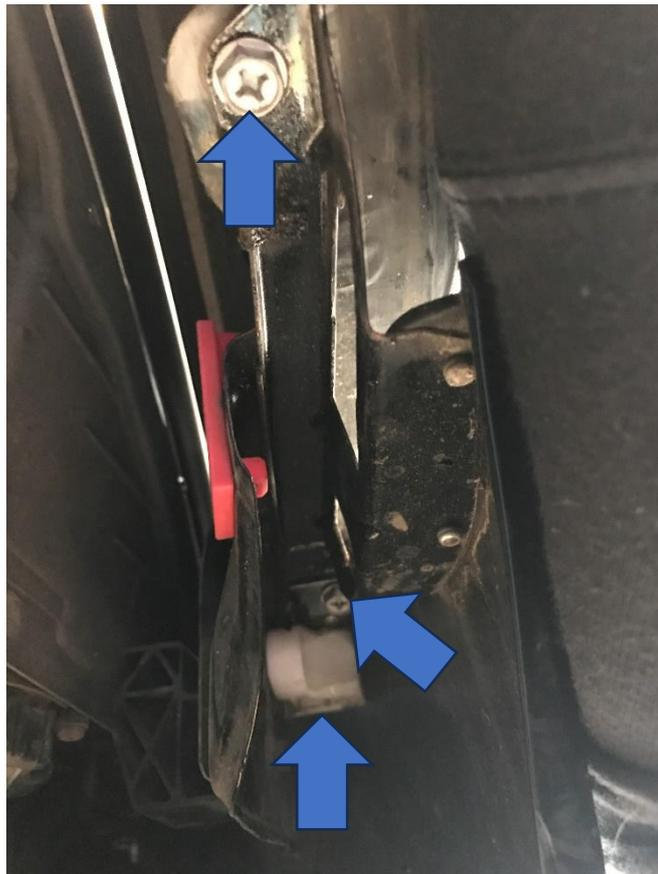
7. Place some protective tape over the bumper and wing and then carefully but firmly pull the corners of the bumper to release them. Then, using the help of a second person move the bumper forward and unclip both the headlight washer pipes inside, as well as the wiring plug above the left-hand side of the crash bar.
