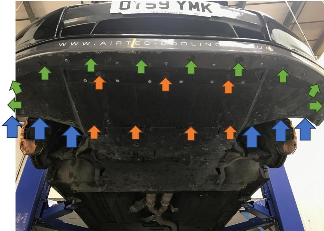
4. Remove the front section of the inner arch liners by removing the one Phillips screw and six push fittings each side.
