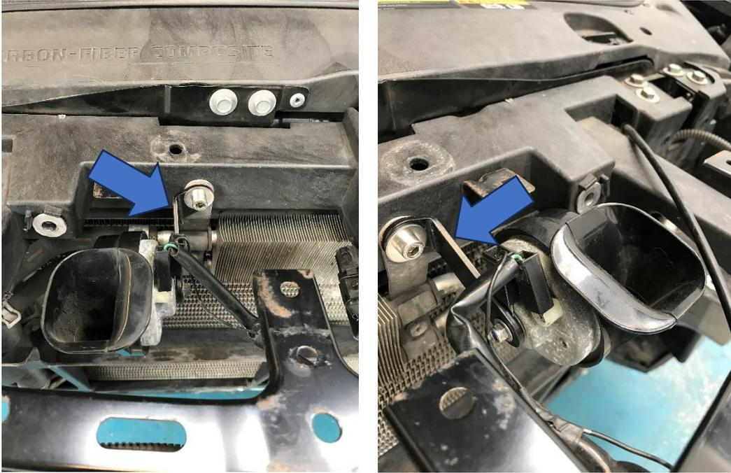
15. Loosely fit both top mounting brackets to the top of intercooler using the supplied bolts and washers.
