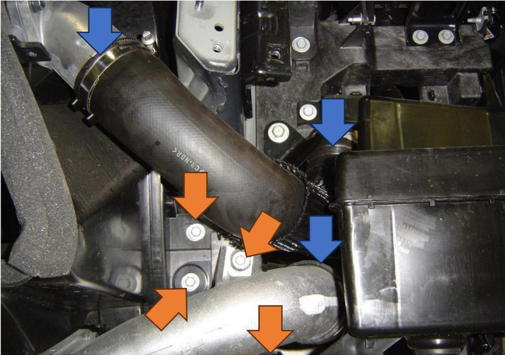
11. Remove the original intercoolers by undoing the two bolts securing the top of the intercooler. Then from underneath, remove the four lower bolts securing each intercooler to the securing frame as well as the single bolt supporting the bottom of the intercooler. The intercoolers can then be removed from the car.
