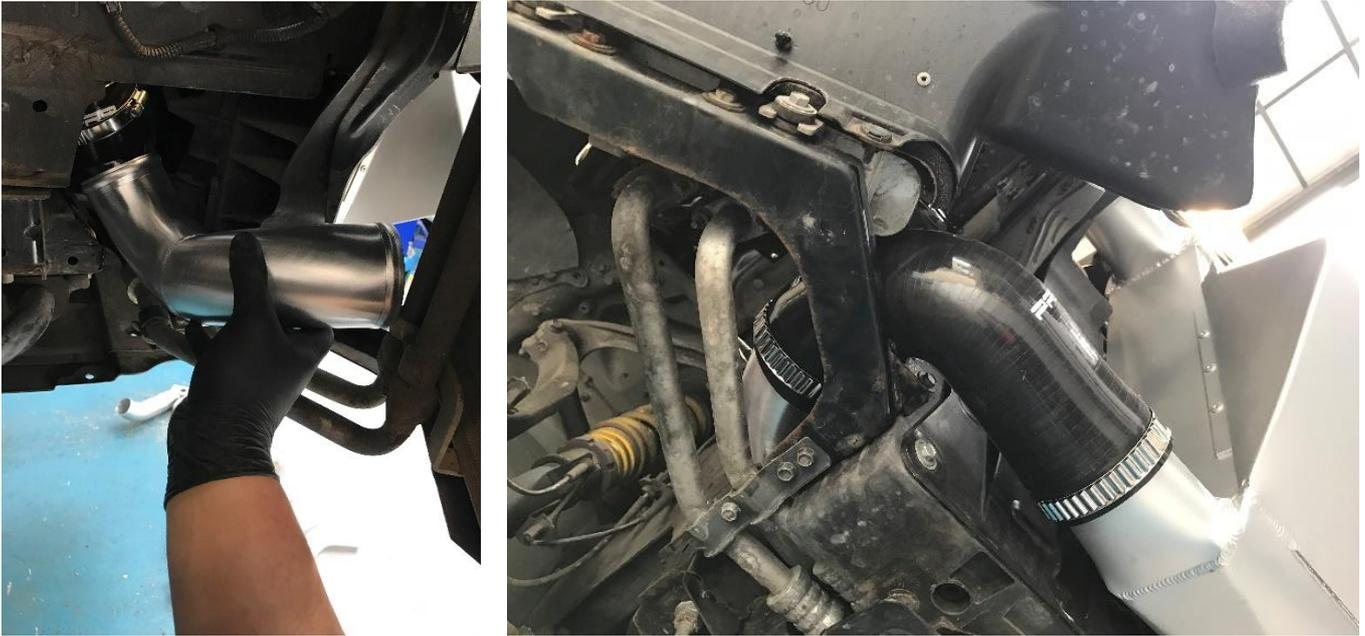
18. Now fit the replacement induction pipes. The driver's side is secured with the original 10mm bolt as shown. Then attach the passenger's side with the original 12mm bolt as shown and attach the filter.
