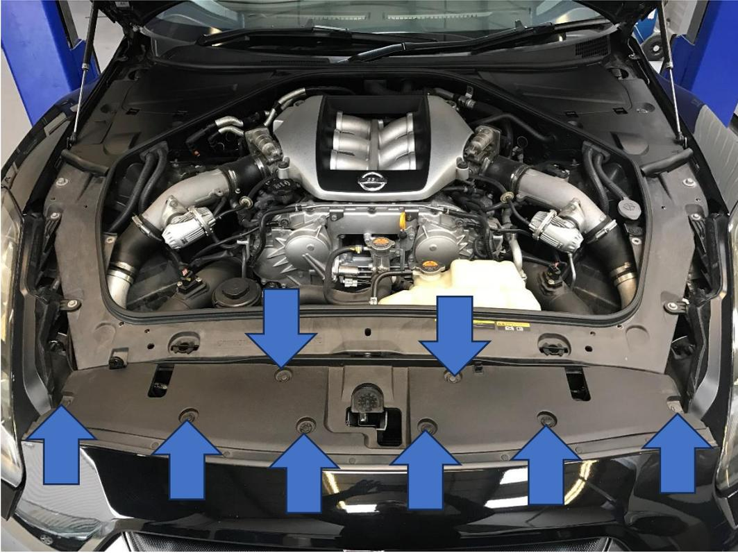
2. Remove the six push fittings securing the top of the bumper.
