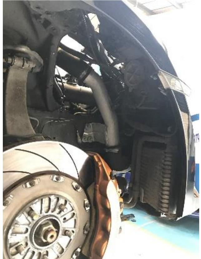
5. Unclip the side repeaters to allow access to the 10mm bolts securing the bumper to the wings.
