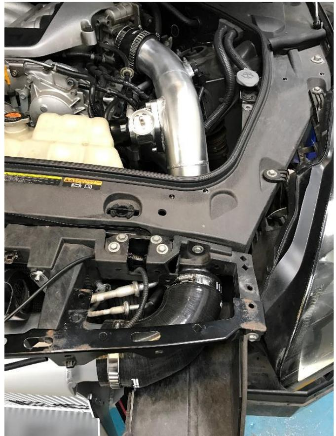
21. Once happy with the location and clearance of all pipes, fully tighten the intercooler mountings.
