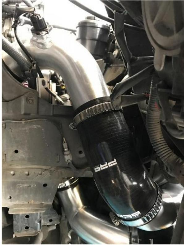
20. Fit the top boost pipes as shown.
