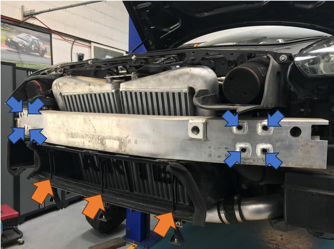
9. Locate the four plastic rivets securing the intercooler shroud in place and cut them off using a Dremel tool or similar.
