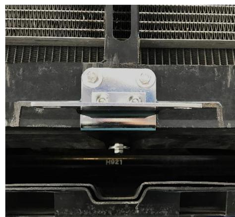
14. Locate the horns mounted on the slam panel and remove them from the original brackets. Then refit them onto the supplied AIRTEC Motorsport relocation brackets using the supplied bolts and washers, as shown.
