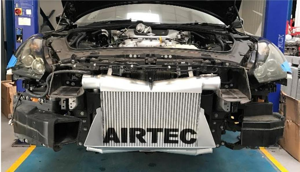
Fit the boost passenger side boost hoses, as shown. Please note: the washer bottle support bracket may require trimming for clearance on the silicone hose.
