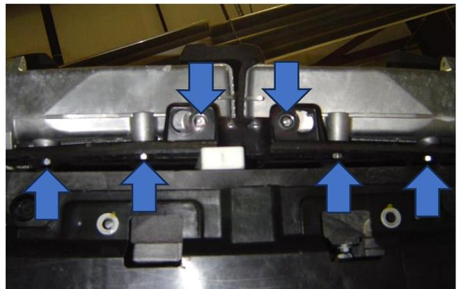
12. The intercooler support frame needs to be cut to fit new AIRTEC Motorsport intercooler, as shown below. Use a Dremel tool or similar and carefully check the clearance regularly.
