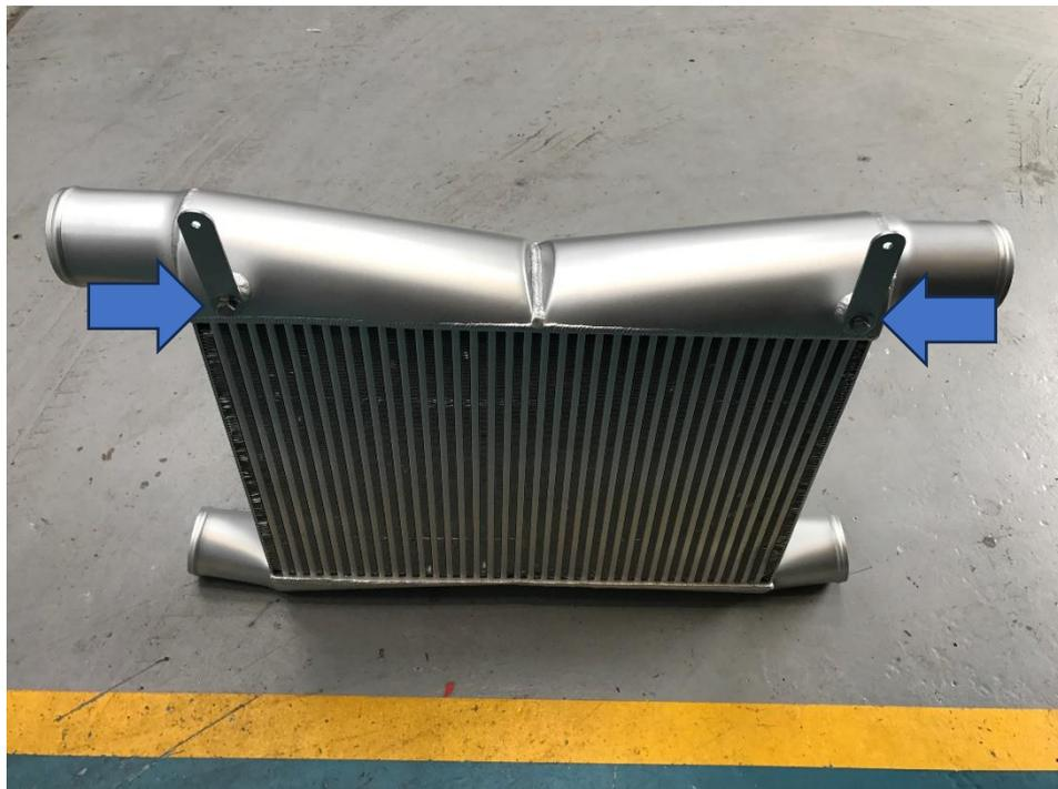
16. Now fit the new AIRTEC Motorsport intercooler loosely into place by locating the top and bottom brackets.
