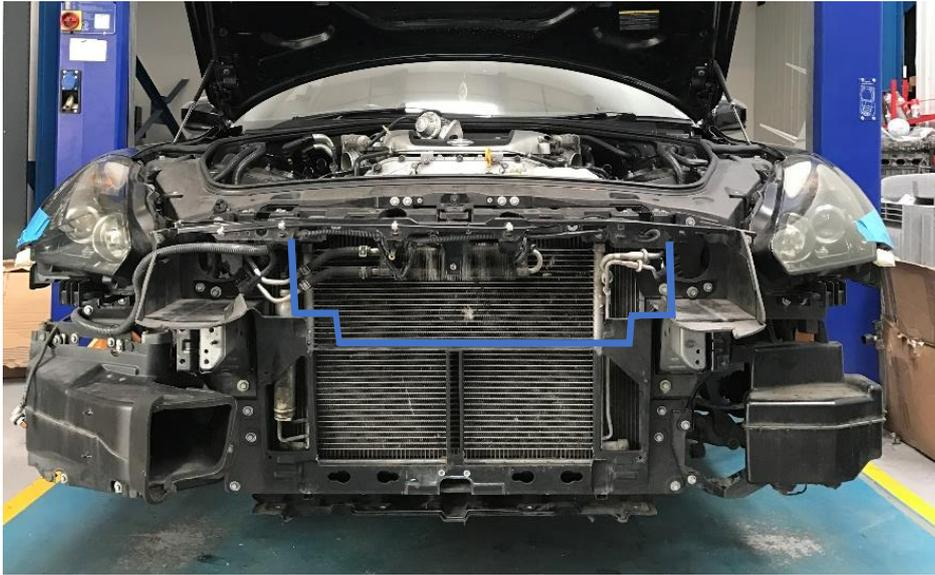
13. The original intercooler lower mounting bracket needs to be removed using a Dremel tool or similar. Then locate the supplied lower intercooler mounting bracket by bolting it from underneath using the supplied bolt and washer (orange arrow). With the bracket in place, mark the two facing holes (blue arrows). Then remove the bracket, drill the holes using a 9mm drill bit, insert the supplied Riv Nuts and refit the lower bracket.
