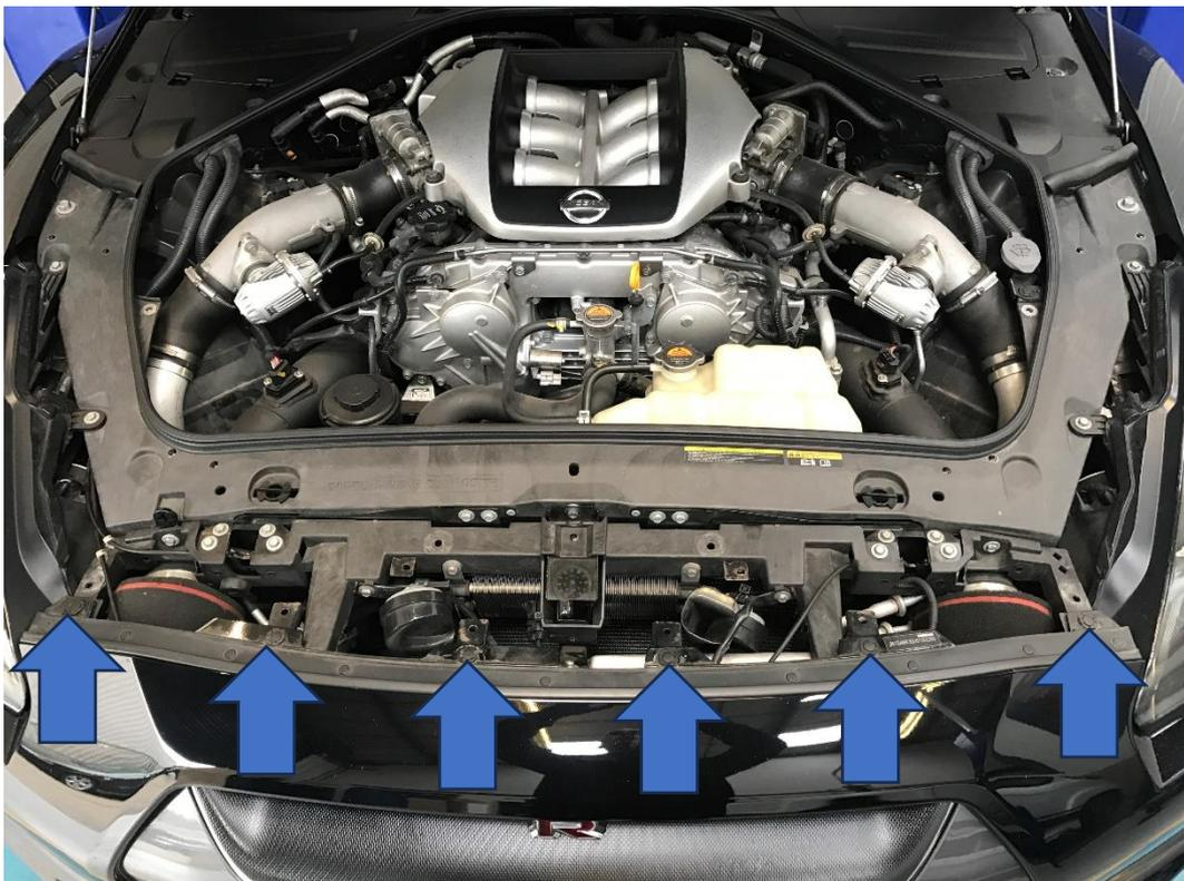
3. Remove the front engine under tray and splitter by releasing the 10 bolts under the rubber grommets (green arrows), the six centre bolts (orange arrows) and the six push fittings (blue arrows) securing it to the inner arches. The front undertray should drop from the bumper and slide out from middle section of the undertray.
