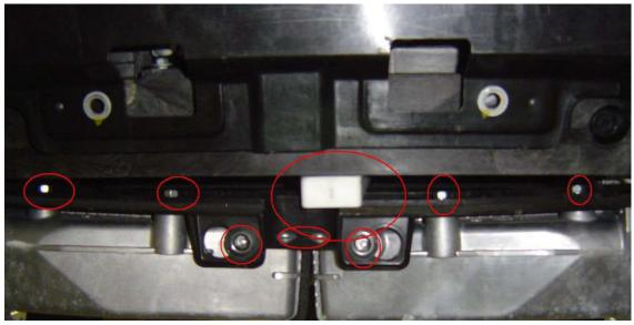
12. Now its time to install the new intercooler as per removal of stock intercooler, install silicone joiners to intercooler and then install alloy bends to silicone joiners and stock boost pipes.
