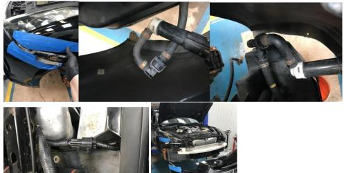
8. Remove crash bar 8x 12mm bolts and 6x 10mm bolts for splitter support bars
