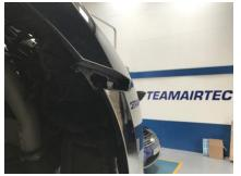
6. Remove 3x 10mm bolts securing bumper to wing
