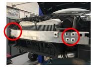
9. Cut 4x plastic rivets securing intercooling shroud and remove shroud
