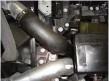
11. Remove standard intercoolers by undoing 2x 12 mm bolts securing top of intercooler, remove 2x 12mm forward facing lower bolts securing bottom of intercooler to securing frame then 1x 12mm bolt securing bottom of intercooler. Repeat for other side intercooler.
