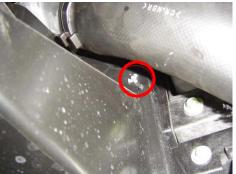
10. Remove all standard boost hoses and induction pipes. Remove 3x 10mm bolts holding intercooler support frame, pull intercooler support away from the car to gain access to hidden intercooler bolts
