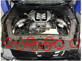
2. Remove 6x push fit fittings securing top of bumper
