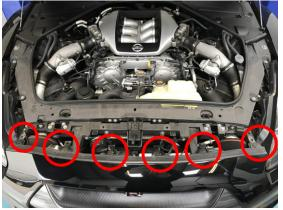
3. Remove front engine under tray / splitter 18 x 10mm bolts & 6 push fit fittings securing to inner arches.
