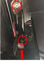
7. Unclip sides of bumper and remove making sure to unclip crash sensor loom and unclip headlight washer pipe
