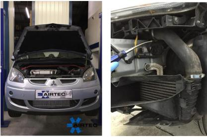
1. Remove front bumper and standard OEM intercooler
