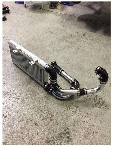
3. Remove front crash bar, install pipework and intercooler into position, re install crash bar to check clearances all okay, tighten and secure intercooler with fixings supplied.
