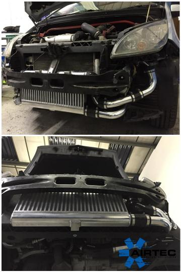
4. Some minor trimming may be required on the back of the bumper
