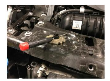
16. Remove 2 x T30 between the radiator cradle and the lower brace.
