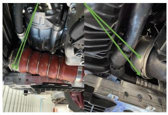
20. Unclip coolant line from the left hand side of the intercooler when looking at it from the front of the car
