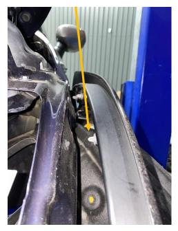
9. Undo 1 x T30 torx each side of the bumper to release from the sides. There is not a lot of space here so ideally you want a T30 torx bit that you can fit a ratchet spanner to which will then allow you to easily remove the bolt.
