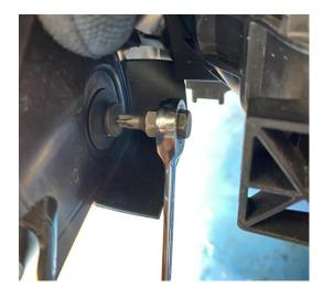
13. Remove 1 x T27 each side to remove the brake duct guides from the car.
