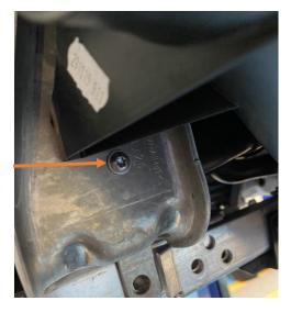
14. Remove 1 x T27 holding the aircon pipework to the right hand side of the intercooler.
