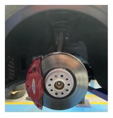
3. Undo the arches by first undoing 2 x 10mm nut and 10 x 8mm bolts each side. 3 of the 8mm bolts are on the underside of the car at the rear of each arch.
