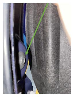
7. The next step is to unclip the front bumper plastic trim from the outer arch, there are 4 clips going along the upright edge and 2 along the horizontal join between the front bumper plastic and the outer arch. These clips need pushing in and then they will release (they may require a little force but be careful not to snap them as they are plastic).
