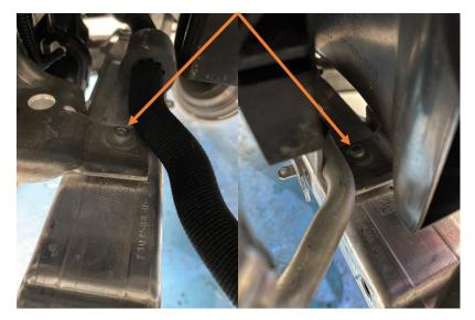
17. Unclip the standard intercooler fixings by using a screwdriver to push down the clip and then pull the black piece down and then remove the centre of the fitting. These can be discarded as they are not needed when fitting your new AIRTEC motorsport intercooler.
