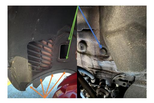
5. Remove the undertray from the car. It separates into 3 pieces, remove the sides first by undoing 4 x 8mm bolts each side and they the tray will pull out, the centre is then held in by 6 x 8mm bolts and will then just come away.
