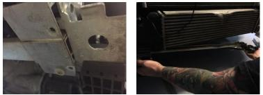
12. Undo t30 from each side of the standard intercooler securing to radiator and remove intercooler.
