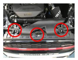
6. Remove plastic speed clip fittings holding brake cooling ducts and inner arch to bumper
