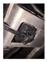
11. Drill out four rivet from the lower rear alloy cross member and remove.
