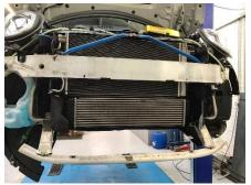
**10.** Unclip bottom of standard intercooler
