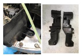
15. Secure intercooler to lower cross member using supplied M8 socket head bolts and washers.
