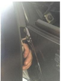
5. Remove 3x T30 torx holding top of bumper to slam panel.
