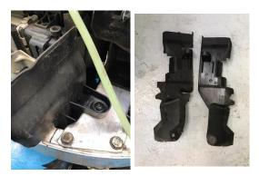
16. Slide intercooler in place between crash bar and radiator clipping in boost pipes. Bolt to original lower fixings and bolt through crash bar to front fixings on crash bar. Once happy with clearance tighten bolts.
