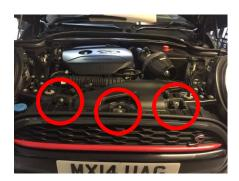
6. Remove plastic speed clip fittings holding brake cooling ducts and inner arch to bumper
