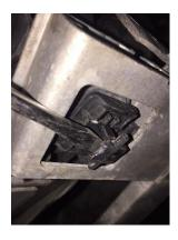
12. Drill out four rivet from the lower rear alloy cross member and remove. PLEASE NOTE: when re-installing please use 4x M6 bolts supplied in fitting kit.
