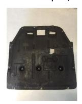
2. Remove 3x M6 bolts connecting M6 bolts to bumper
