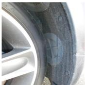
6. Pull wheel arch liner away and then you can gain access to remove the 2 x Push fits from each side, you need to un-clip wheel arches from back using a use flat blade screw driver and then pull forward to release. Once wheel arches are loose you can remove 1 x T25 screw from each side.
