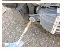
13. The Air temperature sensor is fitted to back of fog light as pictured with cable tie supplied.
