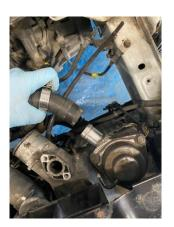
6. Now release the vacuum from the back of the intercooler and unbolt the bracket from the intercooler using a 10mm spanner.
