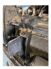
12. The intercooler can now be placed behind the crash bar and the brackets can be secured to the intercooler. Install the right-hand side by using the two supplied M6x16mm Hex Head bolts with M6 mudguard washers, then install the left-hand side using one M8x16mm bolt with an M8 washer.
