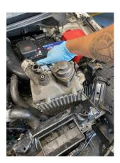
9. The re-circ valve can now be removed from the intercooler using a 10mm socket. You will also need to unplug and unbolt the horn from the crash bar by using a 10mm socket.
