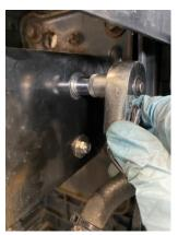
11. Remove the two 10mm bolts from the top of the slam panel then reinstall them with the second intercooler bracket in place as shown.
