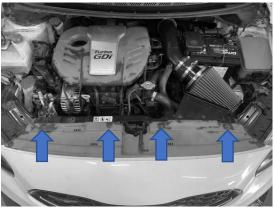
2. Remove your original or AIRTEC Motorsport (pictured here) intake from the engine bay by undoing the jubilee clip and using a 10mm socket and 5mm Allen Key to release the three fixings.
