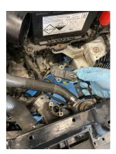
5. Locate the re-circ valve and release the clip securing the vacuum hose to it, then undo the jubilee clip to remove the larger hose from it.
