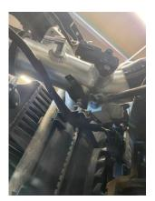
15. The vacuum hoses can now be removed and replaced with the new supplied hoses. Replace the shorter hose with the provided 190mm vac hose and the longer one with the 340mm vac hose.
