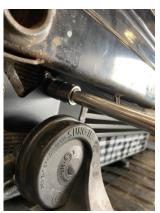
14. Install the silicone hose onto the right-hand side of the intercooler then install the alloy pipework, which the sensor and re-circ valve can also be refitted to. Then secure the other silicone pipe to the throttle body. Also connect the wiring to the boss underneath the alloy pipework by using the M6x12mm bolt with washer.
