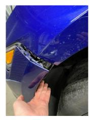
3. Release the undertray by removing the six 8mm bolts and the remaining clips securing it in place.
