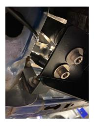
8. Secure the lower tabs of the intercooler by sliding the two supplied Spire Clips onto the lower supports and then secure to the intercooler tabs using two of the original 10mm bolts.
