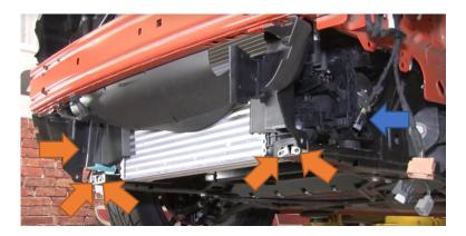
6. Now install the pipework for your new intercooler by sliding the alloy pipe joiners into both original boost hoses and secure using the jubilee clips supplied. Then install the provided silicone pipes onto these pipe joiners making sure the shorter silicone goes to the driver's side (if right-hand drive) and the longer one to the passenger side.
