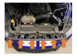
2. Now remove the three trim clips from the arch liner (highlighted with orange arrows) and then firmly but carefully pull the arch liner away from the bumper to access the 8mm bolt securing the bumper to the wing. Repeat this process on the other side and then release the bumper from the wing by firmly but carefully pulling it away.
