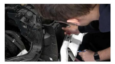
21. Using the second person still get them to align the intercooler so that is level and in the middle. Once happy with the positioning proceed to tighten all of the M8 bolts.
