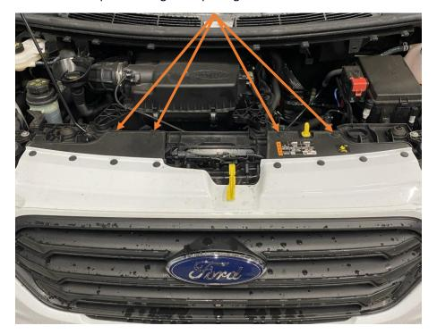
3. Undo the 3 x 8mm bolts also along the top.
