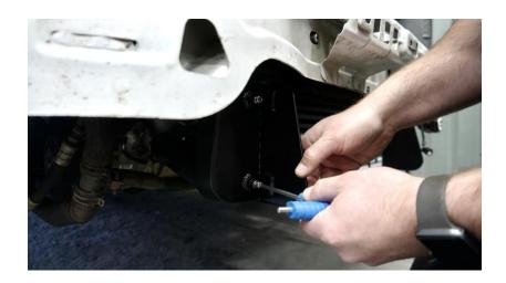
23. Attach the hoses to the intercooler and tighten the jubilee clips.
