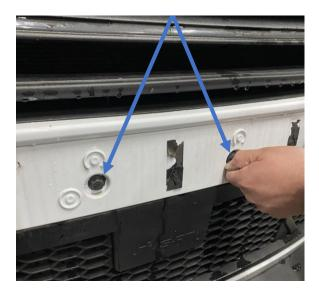
5. Undo the 2 x T27 holding in the headlights and unclip the plug before removing the headlight by lifting it up at the back to clear the tab and then remove from the van.
