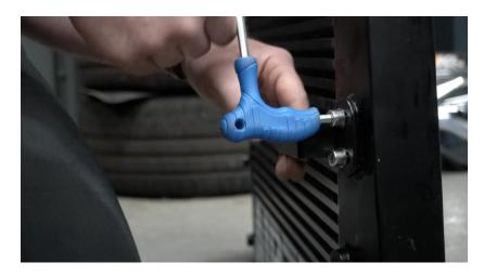
20. Place the provided through bosses in the crash bar and using a second person have them lift the intercooler into place whilst you insert the M8 bolt and then place a washer and nut on and tighten but not fully. Do this for both sides.
