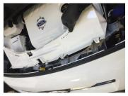
3. Remove push fit fittings holding inner arch to bumper.
