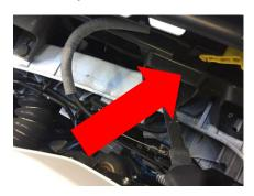
7. Remove bumper, be sure to unclip daytime running lights and ambient air temp
