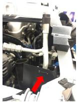
11. Locate intercooler between crash bar and air con radiator taking care not to damage air con rad. Please note: Hoses fitted at later stage, photo for fitting purposes only.
