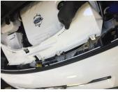
3. Remove push fit fittings holding inner arch to bumper.
