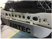
**13.** Drill **2x3mm** holes and cable tie air con pipe into place.
