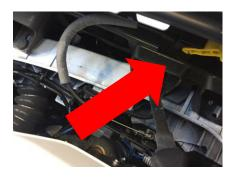
7. Remove bumper, be sure to unclip daytime running lights and ambient air temp sensor.
