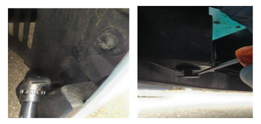
4. Undo the 3 x 10mm bolts securing wing to the bumper (3x bolts each side)
