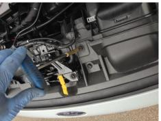
2. Undo 2 x T30 torx bolts on each headlight and remove headlight giving enough room to unclip the multi plug which is located at the bottom
