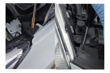
3. Undo 4 x T30 Torx bolts along inner wheel arch liner each side and then remove 2 push fittings along bottom of bumper
