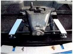
9. Time to attach the side brackets and spacers, this is how the bracket should look just before fitting.
