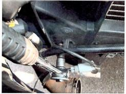
7.Undo the two bonnet catch bolts and loosely attach the two long stainless intercooler brackets
