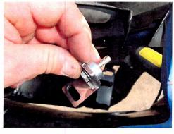
10. The Alloy spacer will fit into the recess of the front panel where you can then loosely tighten the bracket, the slot on the bracket will them line up to the slot on the Intercooler, again loosely tighten.
