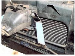
8. Now install the new Intercooler from underneath and loosely connect the two long stainless top brackets, do not tighten at this stage.
