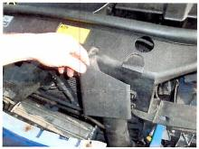
4. To remove old intercooler undo the two 10mm bolts as shown the picture below.
