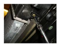
5. Remove original intercooler securing bolts, they are 8mm bolts.
