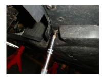
3. Remove both under body splash shields, these are secured by torx 30 screws
