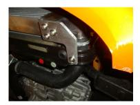
10. Now take the heavy duty 'L' shaped brackets, loosely bolt them on the bottom of the intercooler and radiator support cradle, as seen in picture. Once you are happy with position of intercooler tighten bolts.
