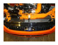
1. Remove main air deflector, located directly behind front upper grill.
