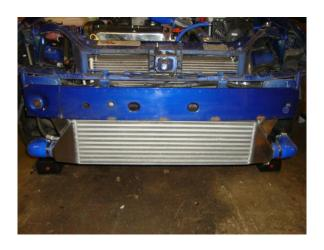
13. Its now time to fit all the alloy pipe work and silicon hoses, we have made this hopefully as easy as possible by labelling all the hoses and pipes with corresponding numbers or positions i.e silicon hose no.6 matches up to alloy pipe no.6 and if its going onto turbo or throttle body it will be marked up 'THROTTLE BODY', there is a picture showing pipe work also. (ONLY REMOVE LABLES WHEN YOU ARE HAPPY YOU HAVE THE PIPES IN THE CORRECT POSITION)
