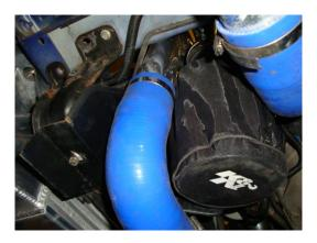
14b. You may need to drill a new hole to mount your k&n air deflector back onto the radiator cradle, please see picture. In your kit you will have longer bolt and machined alloy spacer.
