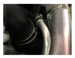
4. Remove 2x T25 bolts securing intercooler into place. Please be aware that this is tight on the plastic air duct, advice trimming the back of air duct.
