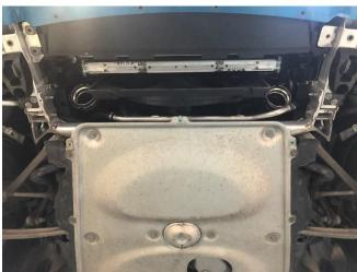
6. Offer the AIRTEC intercooler into place, using the standard intercooler location as a guide. Please make sure to hold back the air guide out of the way to allow as much room as possible, fitting is tight. Tilt the top of the intercooler towards the front of the car, once past the radiator support use the locators on the side of the intercooler to fit into place.
