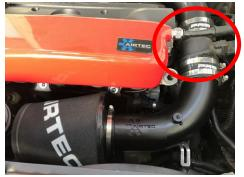
5. Fit air filter to 90 degree hard pipe then fit hard pipe into silicon MAF joiner
