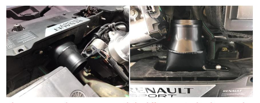
Please note: We have seen some slight differences in the slam panels. Some minor trimming may be required for the pipe to fit.
