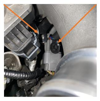
7. Undo the three 10mm holding on the turbo elbow to the turbo. There is a gasket between the two, make sure to not lose this as it will be reused.
