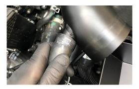
3. Remove the two vacuum lines from the block on top of the induction pipe by squeezing the clips and pulling them back off of the take off and then pull the hoses out of the way.
