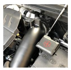
6. There is a clip holding on a plug to the original turbo elbow, using a flat bladed screwdriver, trim tool or pliers remove this clip but leave the plug connected.
