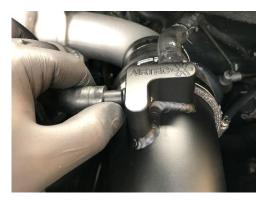
4. Undo and remove the bolt holding the induction pipe to the bracket.
