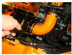
• Fit the new silicone humped step-down hose and stainless Jubilee clips to the air duct as shown. Do not fully tighten any hose clips at this stage.
