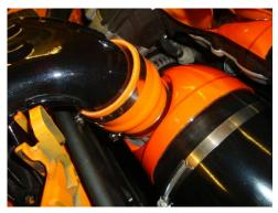
• Make sure you are happy with alignment securely tighten all Jubilee clips and Re-fit Main Air deflector.
