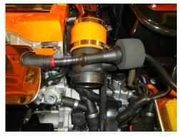
• Then take the 'long' end of the large silicone 90° elbow and connect it to the MAF sensor inlet, then connect the elbow to the CAIS outlet, tighten hose clips, but not fully.
