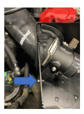
7. You can now install the air filter onto the boss and secure the jubilee clip using a 10mm socket. Check everything is fitted correctly then plug the MAF sensor back in and begin to install the air box lid.
