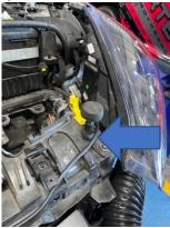
5. Install the MAF boss into the induction pipe using the provided jubilee clip and install your MAF senor in place using a 3mm Hex Key. You will also need to slide the small silicone piece onto the end of the boss in preparation of installing the air filter.
