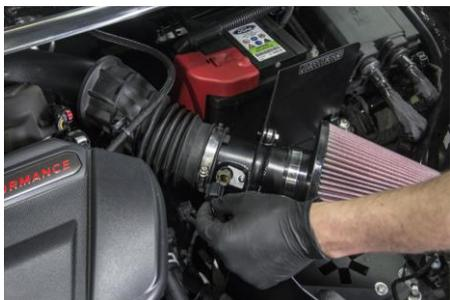
8. Refit OEM air box hose onto MAF housing, making sure all jubilee clips are tight and secure.
