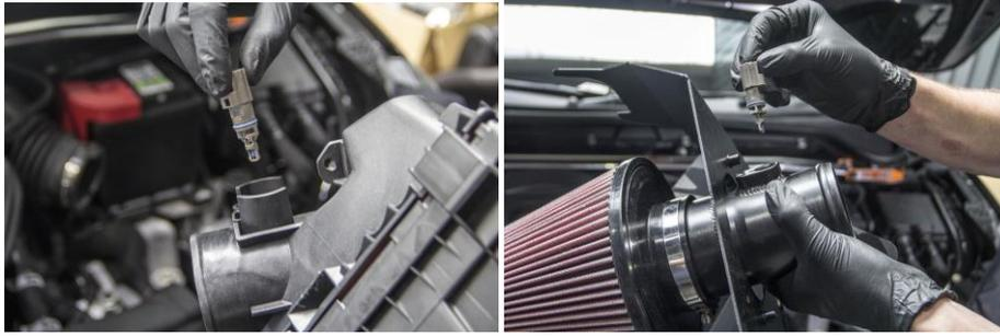
6. Install AIRTEC induction kit into place, locate the 3 pins onto the OEM rubbers, push down firmly to secure.
