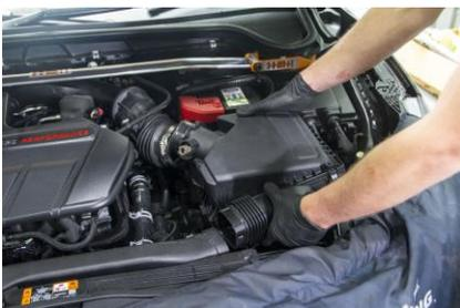
5. With the air box removed, remove the MAF sensor from the air box and fit in to the new AIRTEC MAF housing, using the supplied securing plate to secure.
