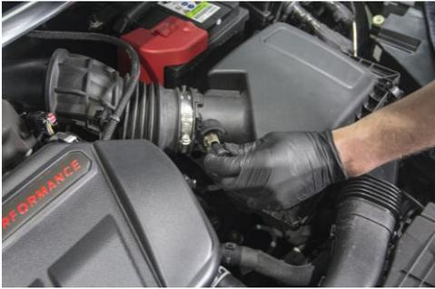
2. With the cable disconnected, loosen the jubilee clips and remove OEM air box hose from standard air box by carefully pulling the hose.
