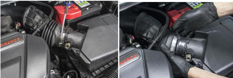
3. Disconnect the standard air box from the cold air feed by pushing the securing tabs to release, using a plastic trim tool or flat blade screw driver to separate the cold air feed from the air box.
