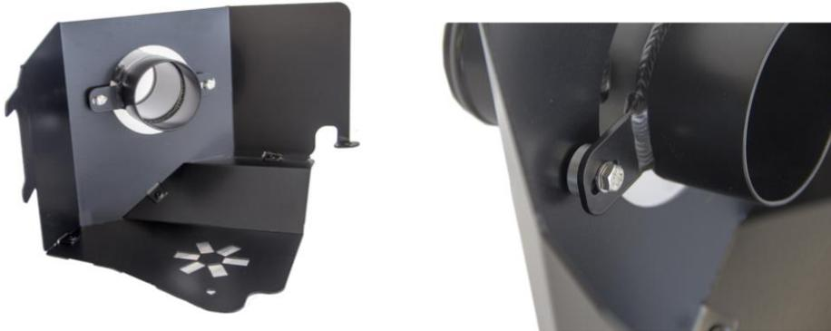
2. Fit the push fittings to the bottom of induction shield as pictured using the 3 x M6 X 16 bolts and 3 X M6 pan washers.
