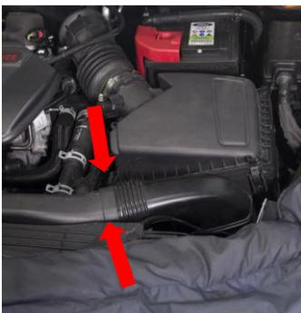
4. With the cold air feed separated, remove the standard air box but giving a firm pull and removing from the engine bay.
