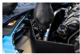
4. Feed new pipe with air filter connected through shield and connect to induction hose then install your original sensor with bolt and washer supplied
