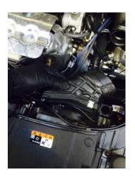
3. Disconnect bonnet catch cable from latch and feed through new shield at the same time install shield into rear locating grommet. Install securing bracket provided onto shield then onto bonnet catch. You'll have to remove 10mm bolt to secure.
