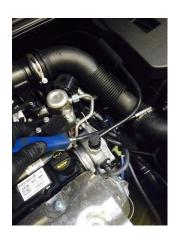
2. Remove airbox (Remove push fit from side of airbox) – pull upwards, also remove rubber intake snorkel
