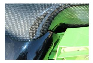
On the rear of the front crash panel there is a lug that sticks out (once you have stage 2 fitted you will see were this is) which on occasion can fail on the side of the stage 2 we would advise removing this with a junior hack saw or file down using a course file.
