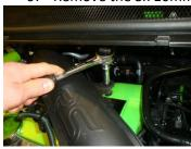
10. Install the silicon hose onto the Airbox outlet and push the Induction pipe at the same time into the silicon hose and place the induction pipe down back into position, replace the 10mm nuts but do not tighten the nuts or the jubilee clips fully at this stage.
