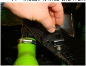
8. Place the carbon Airbox into position in the engine bay, push the machined alloy fitting into the rear rubber grommet
