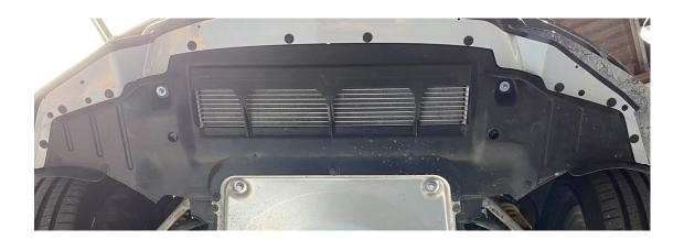
9. The oil level for gearbox must be checked to ensure that it has not gone under level, ensure the car is in the air and is level. To do this firstly remove the middle undertray by undoing 9 x 8mm bolts and 1 x 10mm plastic nut and put the undertray to one side.
