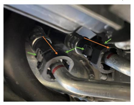
7. Install your new AIRTEC motorsport DCT transmission cooler by clipping in the connector and pushing the on until you hear the positive click of the tabs locking over the collar.
