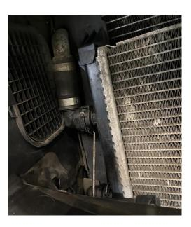
17. The radiator and can then be removed, it is clipped in on the top right so push this clip in and it will come free. It will be full of coolant so best to tip it into a container before putting it down.
