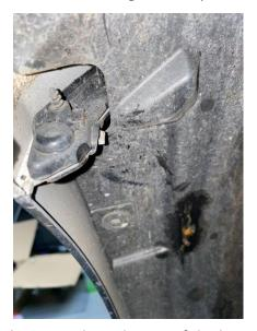
5. Peel back the weather strip along the top of the bumper and remove the  $6 \times T30$  bolts along the top edge.
