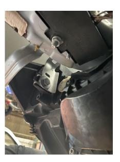
10. The 4 x crash bar bolts can now be removed and the crash bar taken off and put aside.
