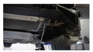
19. Your new cooler will reuse the stock mounting tabs so all you need to do is install in reverse of removal ensuring that the pipework connections are fitted correctly.
