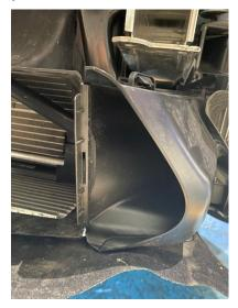
12. Remove the front support brace by unclipping the plastic side air guides from the mouth and removing 1 x plastic pin each side. This step is useful with another person so that they can help unclip the plastic tabs. Then undo 6 x T45 bolts and guide the brace out, be careful when removing to not damage the radiator as it has to tilt towards it to remove.
