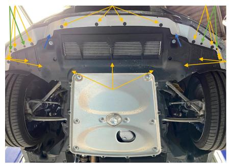
3. The next step is to remove the front half of each inner wheel arch by undoing 8 x 8mm bolts and pulling the front half of the arch liner out.
