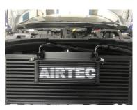
3. Run oil lines from cooler below crash bar into engine bay
