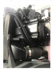
4. Fix oil cooler lines securing bracket to M8 stud on gearbox
