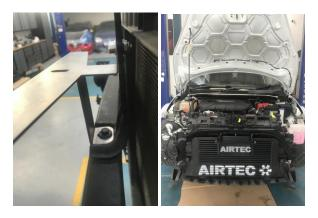
2. Bolt oil cooler to bracket with supplied nuts and bolts
