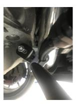
5. Remove standard oil modine and join coolant lines with supplied connector
