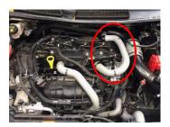
3. Loosely mount breather tank into place using existing hole on manifold, with supplied bolt (no drilling required)
