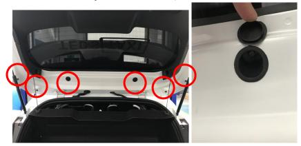
2. Before removing spoiler, remove brake light 2x T20 torx and unclip brake light loom and washer pipe
