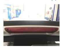
3. Remove spoiler by carefully pulling backwards to unclip from car
