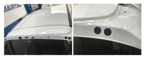
6. Fit spoiler with supplied M6 bolts. Make sure spoiler risers are lined up correctly, once happy with fitment tighten all bolts
