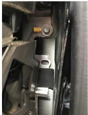
6. For power use ignition live on back of headlight switch
