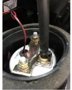
4. Route vac pipe through bulk head grommet and secure onto map sensor take of plate
