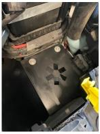
8. Unclip the wiring from where the heat shield will locate using a trim tool then secure the heat shield in place using a plastic trim clip.
