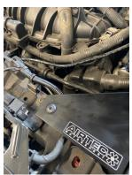
9. Install the vac line onto the fitting coming from the silicone pipework and then remove the MAF sensor from the OEM air box using a T15 and install it into the new housing using the supplied fittings and plug it back in. Finally, attach the new air filter and check that everything is tight
