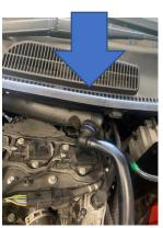
3. Now you can remove the coolant bottle from the engine bay to gain more access to where the crossover meets the turbo elbow. Slide the coolant botte up from the two tabs which hold it in place and once removed loosen the jubilee clip from the bottom of the crossover.
