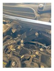
5. Now remove the breather pipe from the engine using pliers and remove the stud securing the engine cover using a 12mm spanner. After it has been removed you can install the larger spacer onto the stud.
