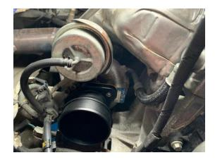
5. Now the reducer has been fitted attach the silicone pipework and secure in place using the provided jubilee clip. Once secured install your new vac hose that has been provided with this kit. Secure both ends of the vac hose with the provided cable ties.
