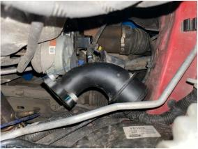
3. Once the elbow and vac hose are removed you can fit the gasket and securing plate to the turbo using x3 Special Machined M6 bolts.
