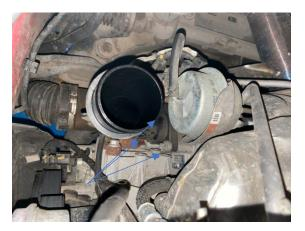
Now you have removed the bolts securing the elbow to the turbo you will now need to disconnect the vac hose from the elbow then follow the hose and remove from the other end.
