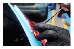
5. Once the hole locations are marked, drill the holes on the boot lid using a centre punch, 3mm drill bit and 6.2mm bit.
