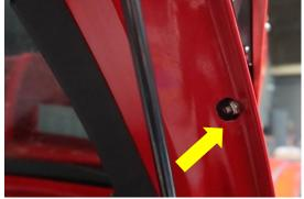
To gain access and tighten the nut on the double skin area of the boot lid, you will need to drill a hole using a 12 - 14mm drill bit.
