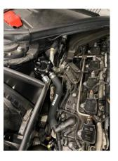
9. Reinstall the turbo elbow in reverse of Step 3. Then install the longer breather hose from the left hand-side of the catch can down to the turbo elbow. Refit the wiring plug and heat blanket removed in Step 3.
