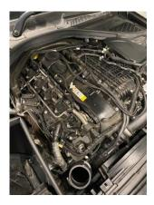
2. Now release the pipework from the top of the cam cover on top of the engine by squeezing either side of the pipe. Then follow the pipe down and unclip the bracket attached to the pipework.
