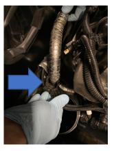
3. You will now need to unplug the wiring connector from the lower turbo elbow. Then remove the heat blanket protecting the wiring by pulling it apart to unclip it.
