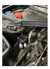
8. Next cut the small plastic tab off from the connecter unplugged in Step 2. Once the tab has been removed, install the shorter breather hose supplied to the right hand-side of the catch can, as shown.
