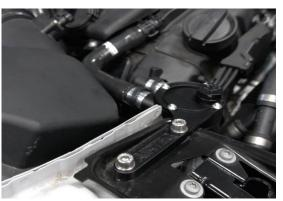
11. Reinstall the strut brace and plastic scuttle covers in the reverse of removal.
