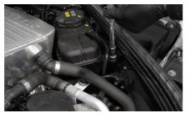
3. The original hose can now be disconnected, one end is connected to the inlet pipe that goes to the forward most turbo. Remove the T25 screw securing the pipework in place and disconnect the plug attached to it. You will now be able to remove this end from the pipework.
