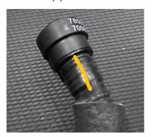
6. The new pipework will need to be assembled as shown below. The end that was connected to the inlet pipe will be fitted to the silicone on the left hand side in the picture below and the other connector to the 90 degree silicone hose.
