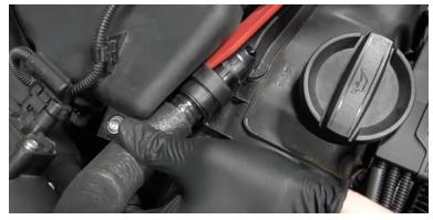
5. After removing the stock pipework, you will need to re-use the stock connections. Carefully use a sharp knife to make a cut down the length of the pipe as shown below and then remove the connectors from the pipe.
