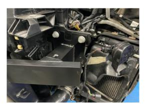
15. Now install the temperature sensor onto the side of the intercooler then clip the wiring onto the side of the crash bar. Install the supplied AIRTEC bonnet latch by reusing the stock 2xT30 screws then use the supplied bolt to secure to the top of the intercooler. Now reconnect the stock boost pipes and check that everything has been fitted and tightened correctly, then finally reinstall bumper in reverse of removal.
