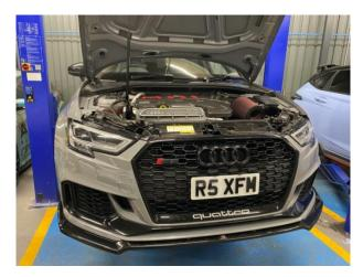
2. Start by removing 3xT30 torx screws securing the slam panel in place.
