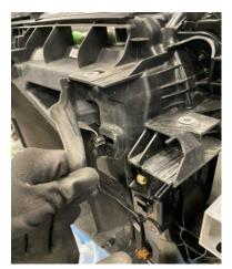
12. Remove all the polystyrene from the bumper by releasing the plastic clips inside them. You will now be able to access the x5 metal clips and remove the 15xT20 screws from the back of the grill then remove the grill.
