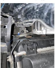
11. You can now remove the crash bar and remove the air guides by releasing the clips from either side.
