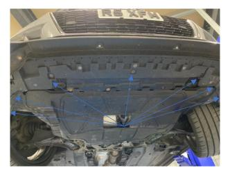
5. Remove 1xT20 Torx screw from the start of the arch liner as shown below to give you access to the 2xT20 Torx screws securing the bumper to the wing and an additional 1xT20 Torx facing towards the front of the bumper.
