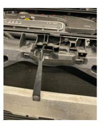
9. Before removing the headlights you will need to remove the bumper brackets located on the wings. Remove these by releasing 2xT30 screws on each bracket then pull away to remove.
