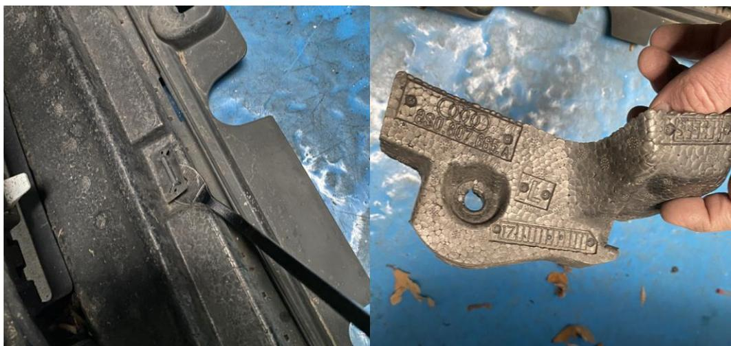
26. Remove the foam section in the centre of the bumper, there is a plastic tube running along the inside of the foam, be careful with this as it is a crash sensor. Remove the tubing from the foam but **do not** disconnect it from either end. The foam is held in place by plastic clips, release the clip and then the foam can be pulled away.
