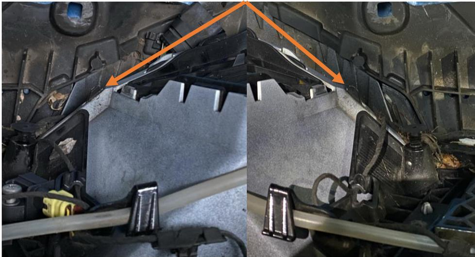
35. Reinstall the bumper in reverse of the removal instructions. When reinstalling the slam panel cover reuse the original clips to install it to the four centre holes but there is no longer brackets for the outer two to clip into however the clips can be pushed back in to make it look complete.
