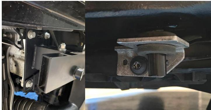
24. Install the air temperature sensor into the bracket on the intercooler as shown.
