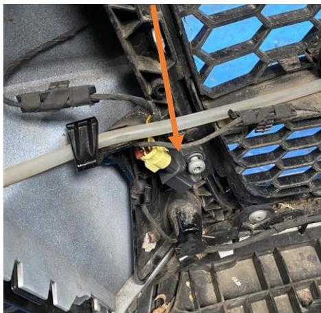
33. Install the four supplied brackets along the top of the bumper as shown reusing the bolts removed when taking the inner frame out, these are used to support the plastic slam panel cover and allows the original trim clips to be reused.
