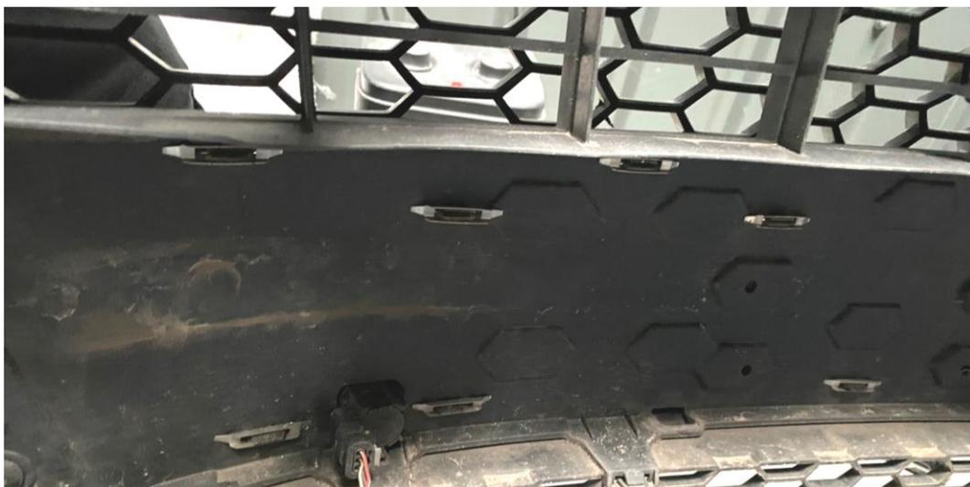
29. Unplug the two parking sensors by pulling the grey tab back and then squeezing the clip together and wiggle the clip apart.
