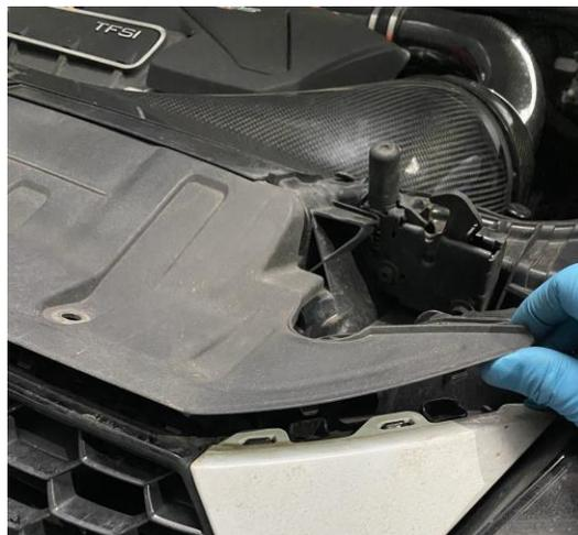
7. Undo the T20 on either side holding the top of the bumper on
