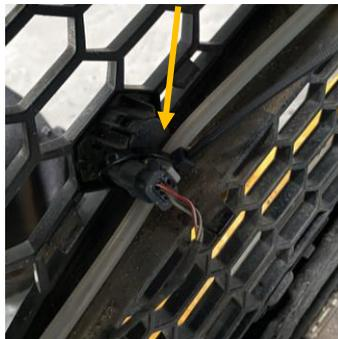
32. Install the sensor as shown in place below.
