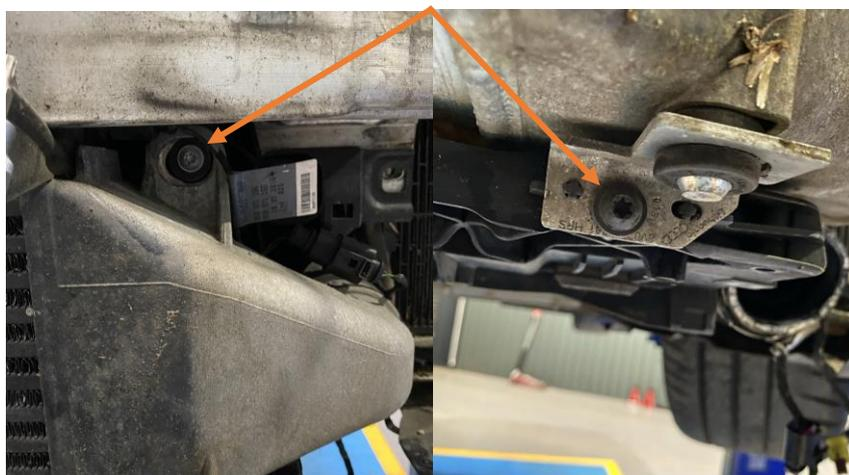
17. Pull the intercooler towards the front of the car to remove, retain the lower intercooler brackets as these are reused when fitting your new AIRTEC intercooler.
