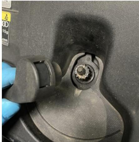
6. The slam panel can now be removed by pulling it from the edges to unclip it.
