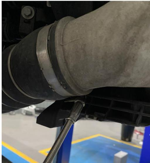
16. Undo the 2 x T25 at the top of the intercooler followed by the 2 x T25 at the bottom holding the intercooler brackets to the car.
