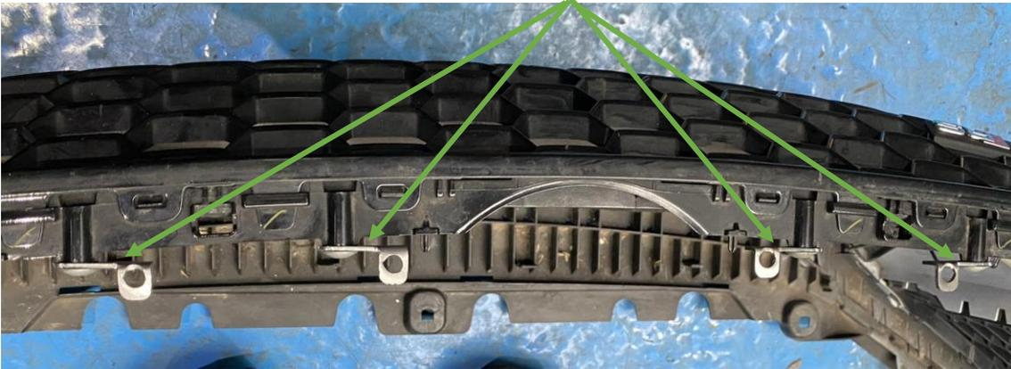
34. The inside of the bumper will also need slight modifications in the lower corners in order to clear the inlet and outlet pipe on the intercooler. Using a sander or angle grinder lightly trim both sides where the clip comes through until it is flush, if it is tight when refitting the bumper then remove more material at these points until happy with the fitment.
