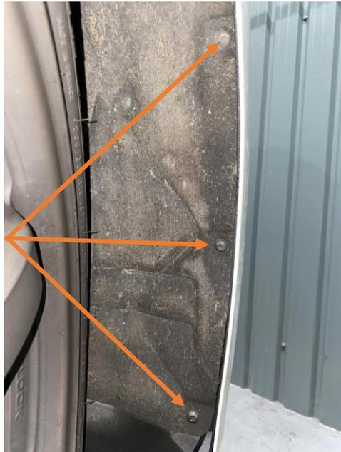
9. Undo the T20 holding the bumper to the wing in each arch
