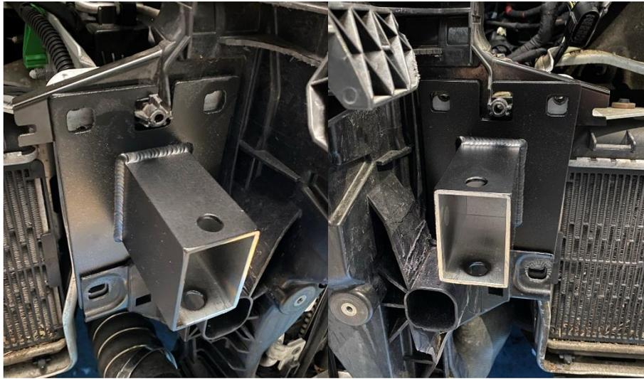
21. Fit the original lower mounting brackets from the stock intercooler on to your new AIRTEC intercooler. Using a second person place the intercooler and crash bar assembly onto the car, insert the two supplied M12 bolts with washers from the bottom through the crash bar foot and intercooler assembly and then use the other supplied M12 washer and nut on the top and tighten.
