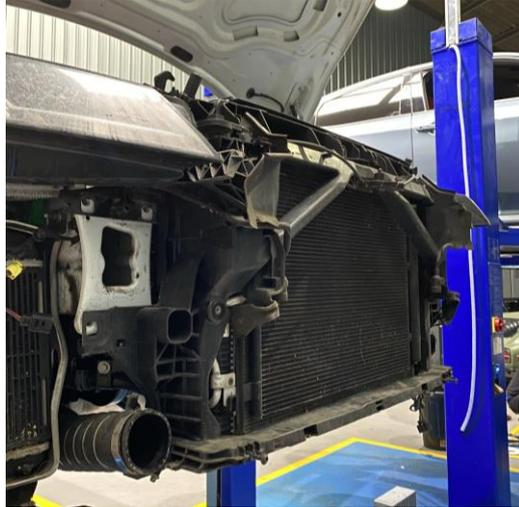
19. To fit the new intercooler you will need to modify the plastic rad pack surround, see the marks on the photo below and using a sander or angle grinder remove material. Be very careful to not catch any pipework to the air conditioning condenser. Start by removing a small amount of material in that area and then lining up the intercooler to check clearance and then remove more as needed.
