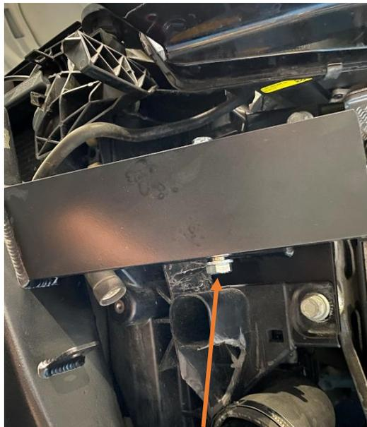
22. Once the intercooler is in position attach the stock hoses and tighten.
