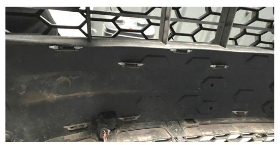
24. Unplug the parking sensors by pulling the grey tab back and then squeezing the clip together and wiggle the clip apart.
