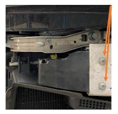
12. Remove the ducting to the auxiliary coolers, It is held in by plastic clips. The top needs to be pushed down slightly to release before it can be pulled out. Take care as the clips can be fragile. On the right hand duct there is wiring attached to it that will need to be unclipped using a trim tool or similar.
