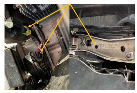
13. Unplug the horn and crash sensor wiring on each side and push the wiring clip through to release the wiring from the bracket.
