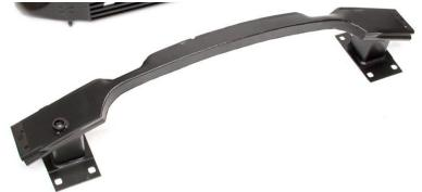
31. Using a second person to help you guide the crash bar onto the car, you will need to tilt it back first to get it past the front of the rad pack and then tilt it forward to get the bottom to slot in behind the rad pack. Once in position reinstall the original crash bar bolts and tighten the lower mounts.
