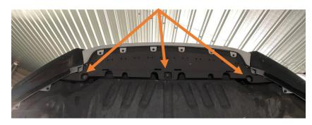
4. Working from the top now, use a trim tool to remove the 6 x slam panel clips
