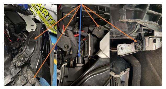
27. Before it can be removed you will need to undo the brackets that hold the bumper to the wing, undo the 2 x T27 each side and remove the bracket from the car.
