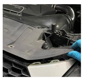
7. Undo the T20 on either side holding the top of the bumper on
