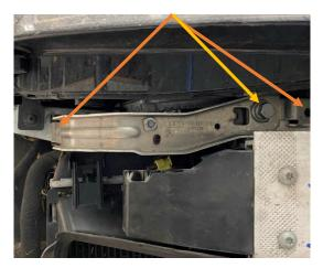
15. To remove the intercooler firstly loosen the two jubilee clips using a 7mm flexidriver or socket.
