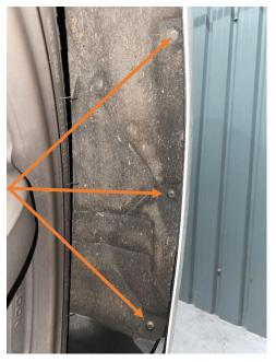
9. Undo the T20 holding the bumper to the wing in each arch
