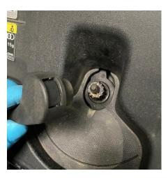
6. The slam panel can now be removed by pulling it from the edges to unclip it.
