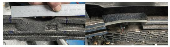
22. If you want maximum airflow to the intercooler then you can remove the centre blocked off section of the front bumper and remove the foam centre section entirely which means you will not need to cut it however this is an optional step, this is done by undoing the T25 torx bits along the top and the bottom, then remove the two T25 torx bolts holding the sensor bracket, then unclip the wiring that goes along the top of the bumper and lay the sensor aside.
