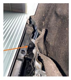
10. Using a second person at this stage pull the edges of the bumper away from the wing to release it, with the bumper pulled forward slightly get the other person to disconnect the plug connecting the wiring from the bumper to the car. Put the bumper safely aside.
