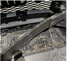
18. Now remove 16 T20 Torx bolts holding in the rear plastic support (four along the top, four each side and then four along the bottom). Once undone pull from both sides and it will release.
