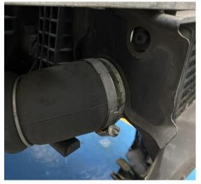
9. Unbolt the top of the intercooler by undoing the 10mm bolt on each side.
