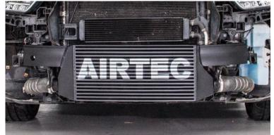
You can now refit the bumper to the vehicle, however we recommend for increased airflow and maximum performance to follow the below steps to remove the centre section of the grille that blocks some of the airflow.
