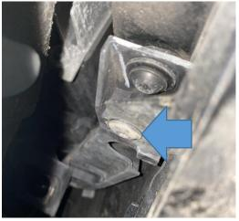
8. The original intercooler and crash bar can now be removed. Start by loosening the jubilee clips on the intercooler hoses and remove them.
