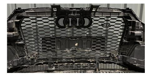
21. Finally, the bumper can then be reinstalled in the reverse of Steps 2 to 7. Please note; when reattaching the arch extension removed in Step 6 you may need to lift the back corner of the bumper over the inner lip to get the clips to fully seat home.
