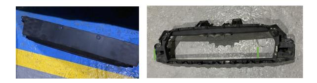
20. The surround can now be reinstalled using 14 of the original fixing to hold it in place.
