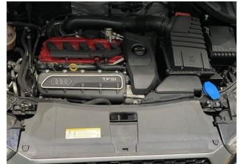
2. Remove the front upper panel by lifting at the edge and then pull the panel out.
