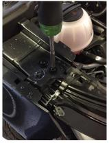
**12.** Unclip bonnet catch sensor clip x2 L/R from crash panel.
