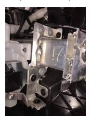
**11.** Remove 4x T27 from slam panel & top of engine bay.
