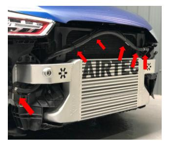
21. Before installation of the new AIRTEC intercooler, you will need to trim the plastic radiator surround.
