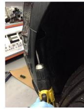
5. Remove T30 bolt in each arch and remove bumper.
