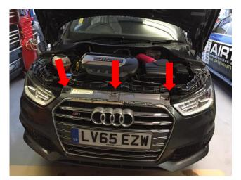
2. Remove 3x T20 torx on inner arch to bumper, 1x push clip inner arch to bumper (pull inner arch liner back).
