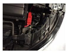
8. Remove 1x T30 torx below headlight to drop headlight washer cradle down.
