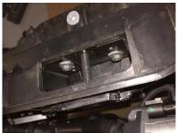
16.Undo 2x torx from crash bar to rad and unclip sensor from plastic surround.
