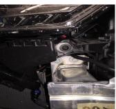
9. Unclip washer jet & air temp sensor and move to the side.
