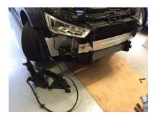
10. Remove 7x T30 from rad pack to slam panel, remove horns from O/S.
