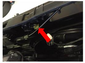
15.Unbolt 3 bonnet catches and slide out & lay across engine 6x 10mm bolts.
