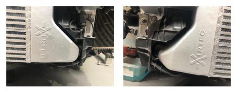
22. Install AIRTEC intercooler into place securing using original crash bar fixings, fit original boost pipes onto your new AIRTEC intercooler.
