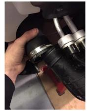
20. Remove original washer jet pipe that runs along the top of original crash bar, one end unclips and the other end depending on the year of vehicle will possibly need to be cut off. Install new longer washer hose with supplied jubilee clips and cable ties (Please see photo below). When you install the new AIRTEC intercooler, please check the pipe does not get kinked or caught upon installation.
