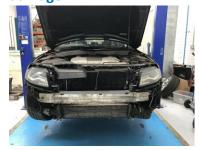
6. Remove standard cooler by removing boost pipes. Undo 1x T25 on passenger side and unclip cooler.
