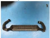
7. Fit new airtec intercooler into place. The bottom sits into original mounting points and secure top of cooler to crash bar with supplied bracket.
