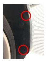
4. Undo 10mm bolt securing bumper to inner wing, then unclip side of bumper
