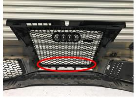
13. Refit bumper and check clearance between grill and cooler, following instructions in reverse.
