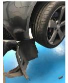
3. Undo 1x T20 torx securing bumper to arch
