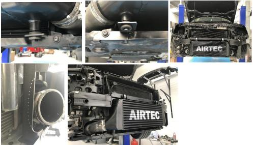
12. Before re-fitting bumper, lower section of grill will need minor trimming to fit
