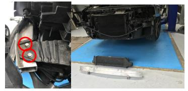
11. Fit new AIRTEC intercooler & modified crash bar into place with supplied lower brackets.
