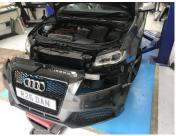
8. Remove standard intercooler undo both boost pipes 10mm bolt each side securing to crash bar and T27 torx securing bottom brackets
