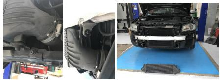
9. Remove headlights 3X T27 Torx & 2x T27 torx securing headlight washer housing
