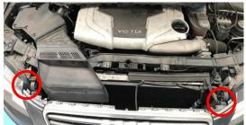
3. Undo 2x T25 torx securing inner arch to bumper
