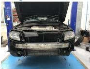
6. Remove standard cooler by removing boost pipes. Undo 1x T25 on passenger side and unclip cooler.
