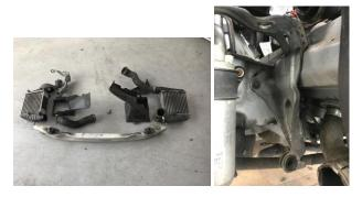
10. Re locate horns, these need to be fitted to front radiator housing underneath headlights as pictured
