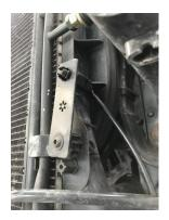
12. Power steering securing bracket needs to be removed in preparation to fit intercooler
