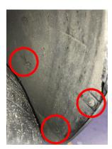
4. Remove 2x T20 torx securing lower bumper
