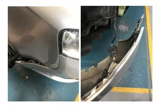
7. Remove intercooler air feed guides by simply unclipping and remove
