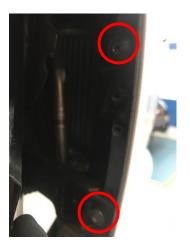
5. Remove 2x 10mm nuts securing bumper to inner wing
