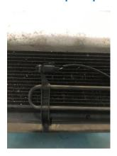
9. Remove both standard intercoolers pipework and securing brackets and crash bar
